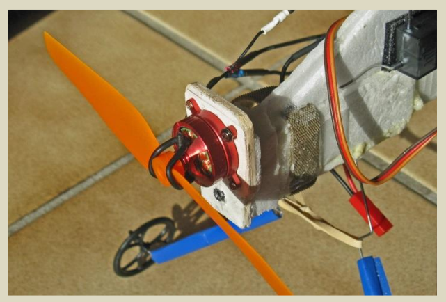
AEO 16 g (1904?) motor on rebuilt nose of Gym Stik
