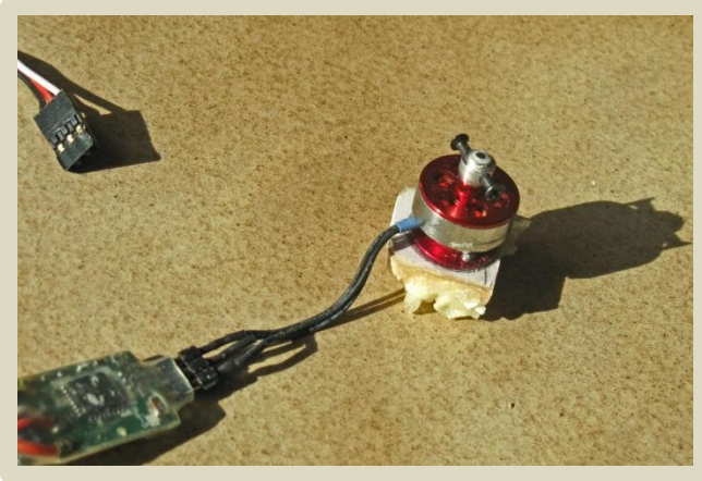
AEO C10 (8 g) Motor with factory 5A ESC
